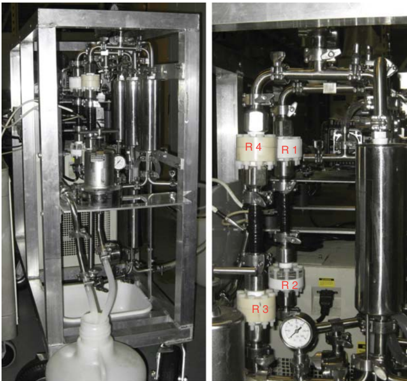
Figure 9.5 Small pilot scale CHIEF system with four treatment chambers/reactors (R1, R2, R3 and R4).
