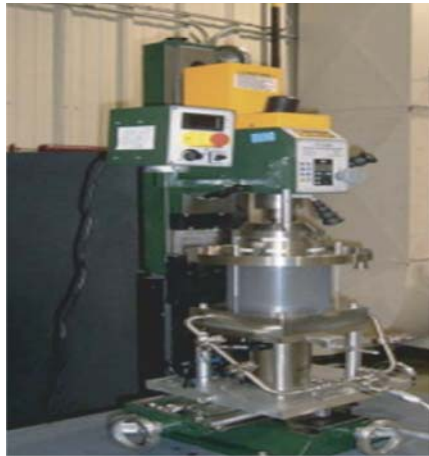
Figure 7.3 Taylor–Couette UV reactor. Gomez-Lopez et al. , 2010. Reproduced with permission of Elsevier.
