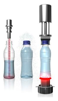
Figure 9.4 Base re-heat diagram (courtesy of Plastipak).
