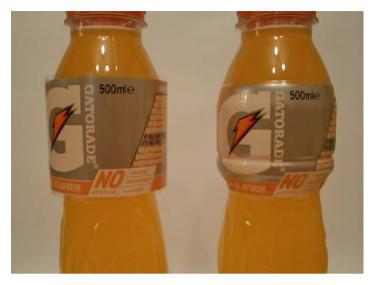
Figure 9.13 Shrinkable label, as applied and shrunk to a bottle (courtesy of Britvic Soft Drinks Ltd).
