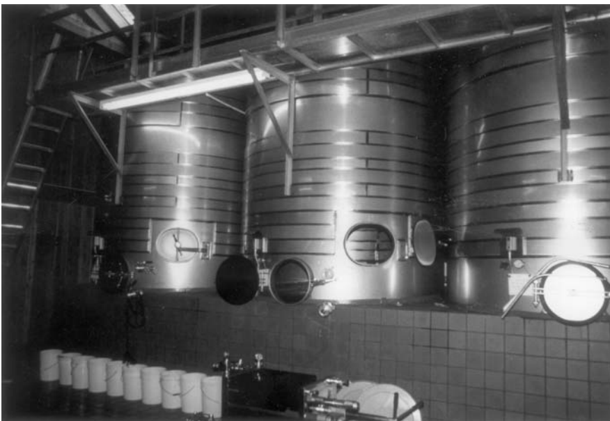
Figure 20–1 Red wine fermentation tanks. Courtesy of Bruce Zoecklein, Virginia Polytechnic Institute & State University, Blacksburg, Virginia.
