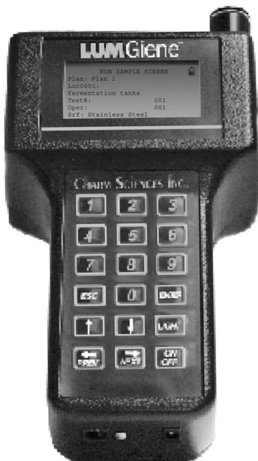
Figure 3–4 Device for the rapid determination of hygienic conditions.
