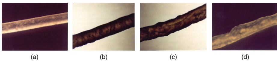
Plate 12.13 Microscopic observation of rice noodle (diameter 0.6 mm) surface prepared by direct extrusion cooking (a) and commercial products prepared by conventional process (b-d). Source: Adapted from Charutigon et al. , 2008
