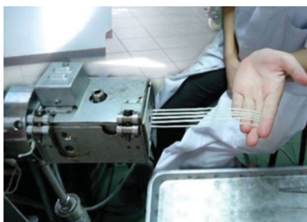
Plate 12.14 Direct extrusion of rice noodle (flat type) from rice flour using a laboratory single screw extruder (Brabender 19/20 DN Model Do-Corder DCE 330, Germany)
