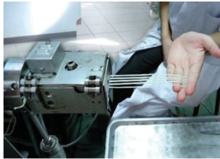
Figure 12.14 Direct extrusion of rice noodle (flat type) from rice flour using a laboratory single screw extruder (Brabender 19/20 DN Model Do-Corder DCE 330, Germany). For colour details, see the colour plates section
