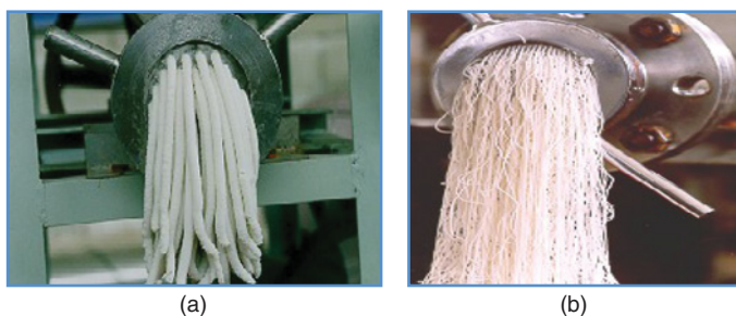
Figure 12.11 Extrusion of rice cake (a) and after pregelatinized by steaming (b) in most conventional method for rice vermicelli production. Source: Yoenyongbuddhagal, S. (2002). The effects of processing condition on ricevermicelli quality, Dissertation No. PH-02-2, Food Engineering and Bioprocess Technology Program, School of Environment, Resources and Development, Asian Institute of Technology, Thailand, 140pp. For colour details, see the colour plates section
