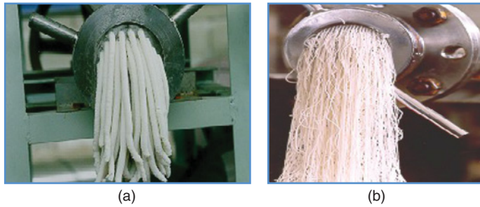
Plate 12.11 Extrusion of rice cake (a) and after pregelatinized by steaming (b) in most conventional method for rice vermicelli production. Source: Yoenyongbuddhagal, S. (2002). The effects of processing condition on ricevermicelli quality, Dissertation No. PH-02-2, Food Engineering and Bioprocess Technology Program, School of Environment, Resources and Development, Asian Institute of Technology, Thailand, 140pp
